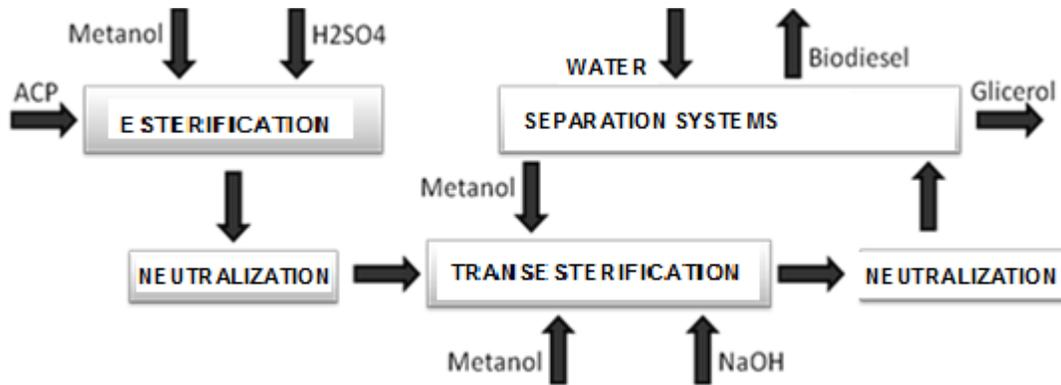
Figure N° 1. Technological Scheme of Biodiesel production using Palm oil
